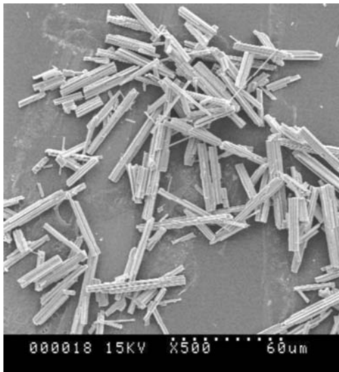
Fig. 7 A SEM micrograph of \text{KSr}_2\text{Nb}_5\text{O}_{15} particle powders synthesized at 1150^\circ\text{C}
